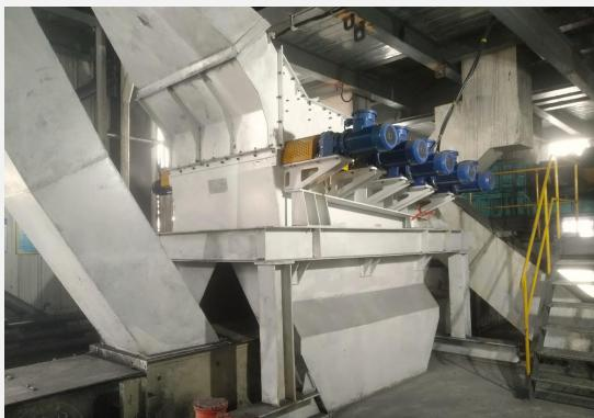
The coal fines deep classification roller-disc screen can be used for raw coal desliming to reduce the load of slime water and improve the overall treatment capacity of coal preparation plant.
